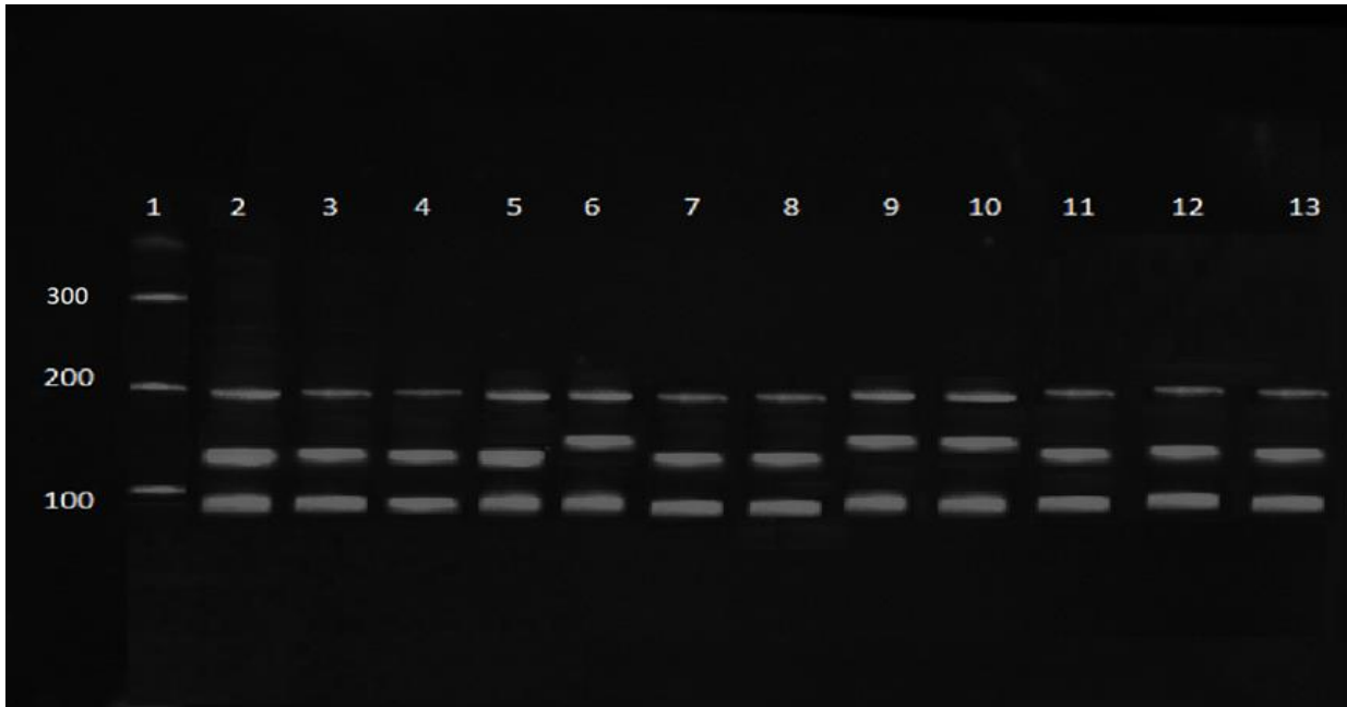
Figure 1. PCR-RFLP profiles of the gyrA gene using TaqI restriction enzyme. Lanes 2, 3, 4, 5, 7, 8, 11, 12, 13 for KpI (197 bp, 142 bp, 93 bp, and 9) and lanes 6, 9, 10 for KpII (197 bp, 151 bp, and 93 bp) . Lane 1, 100 bp molecular DNA marker (Axygen Biosciences).
