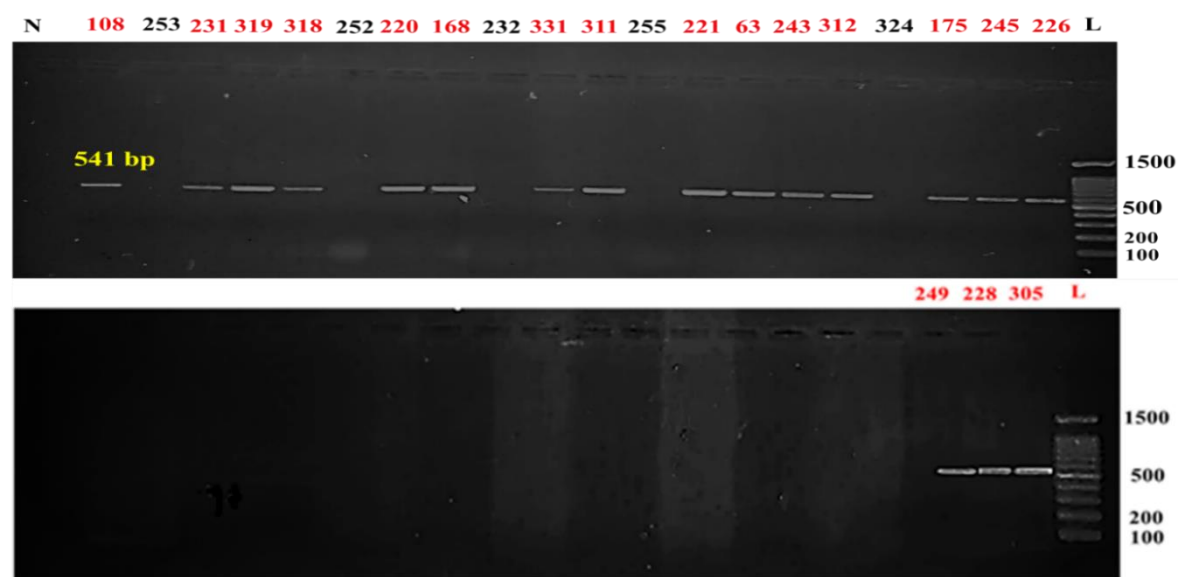
Figure 5. Agarose gel electrophoresis of Class 1 integron gene amplified from 19 MBL producing A. baumannii isolates using 100 bp DNA marker. N: negative control, L: ladder
